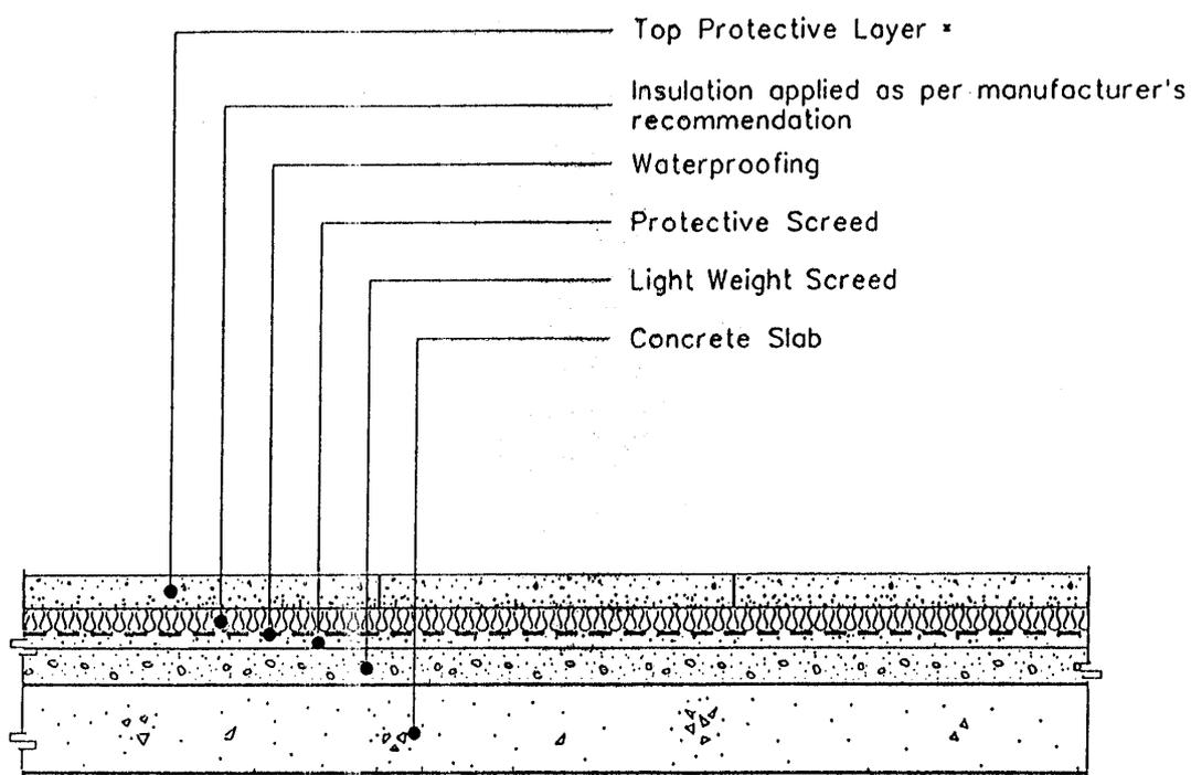
\* - As per the Arch./Eng. recommendation (Paving slab, terrazzo tiles, stones balast, etc.)
