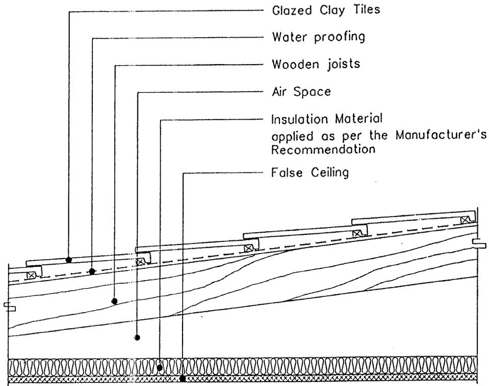
\* - Recommended for existing building with no insulation incorporated at the roof
